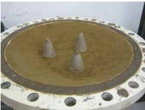
Figure 6. Truncated cones used for testing on subgrade
