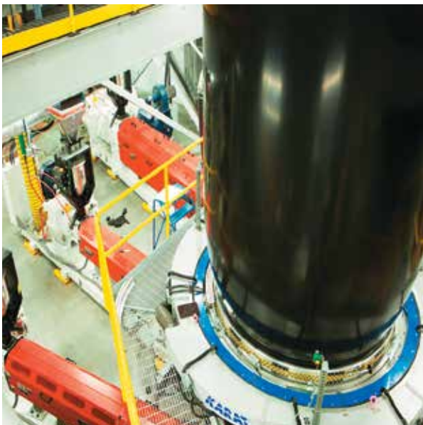
Figure 2. Layfield's Line 9, a wide width geomembrane manufacturing line.
