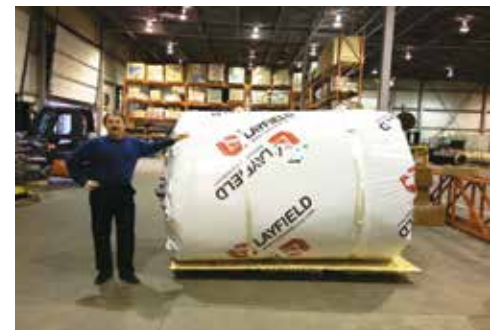
Figure 14. 7000 lbs (3200 ks) one-piece prefabricated Enviro Liner® 6030
