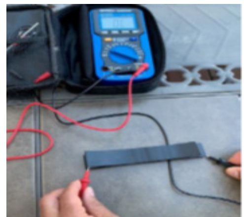
Figure 4. Using ohmmeter to qualify conductive side
